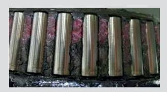
The red lithium-complex grease that Austrian Airlines normally uses, which does not meet the SAE AMS 3058 specification, after 548 cycles shows:
